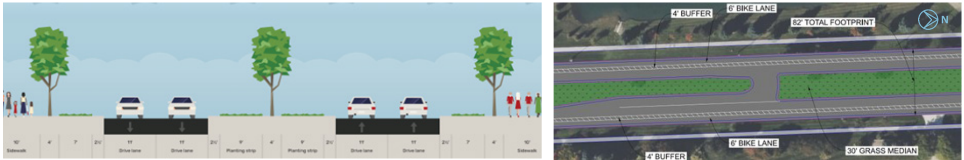
Figure 18: Alternative 5 Typical Cross-Section and Aerial View
