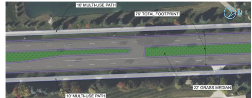
Figure 17: Alternative 4 Typical Cross-Section and Aerial View
