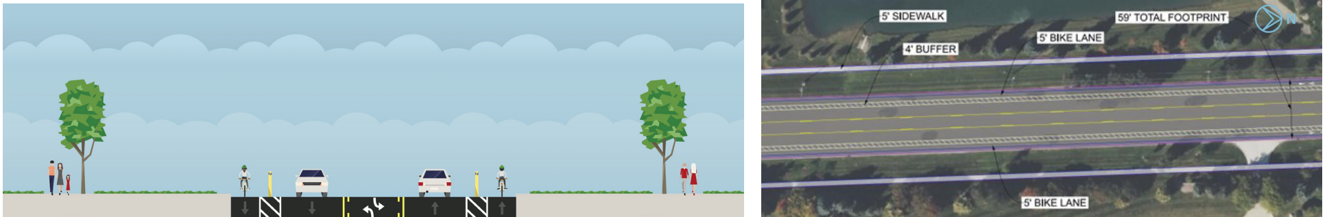
Figure 15: Alternative 2 Typical Cross-Section and Aerial View
